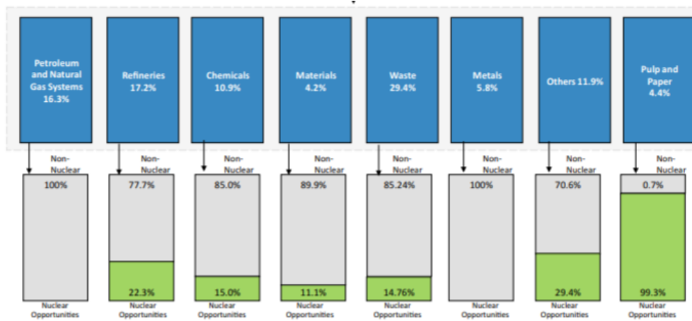
Figure: Share opportunities for waste heat integration by industry from nuclear power plant. The green area represents low temperature heat sink opportunity, and by corollary the grey represents a potential heat sources.
